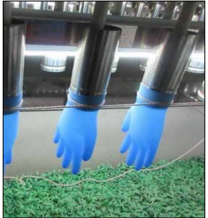
Water Leakage Check
